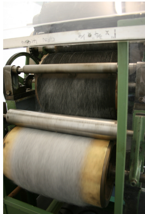
Fig 68 Carding machine showing web formation
