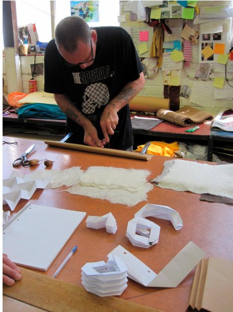
Fig 94 Scoring new pattern template at Ciment (pleating) Ltd.
