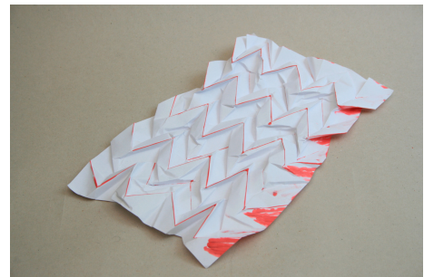
Fig 93 Pressed template [Fig 92]. Red marks identify the chevron pattern in a two-dimensional plane.
