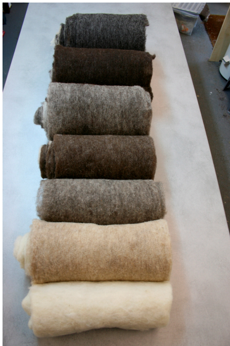
Fig 67 Machine carded batts of British wools
