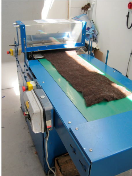
Fig 69 Needle punch machine with carded web of Zwartbles (ZB)
